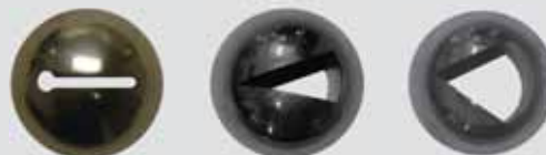
V-ports 15, 30, 60, 90 deg V & slotted balls.
