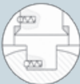
Pyramidal Stem, Double Sealing & Anti-Static Device (Optional)
